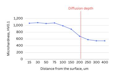
• Example of H13 tool steel after Ion Nitriding - surface hardness and diffusion depth
